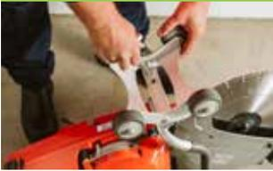
1. Remove the rubber feet from the base of your demolition saw.
