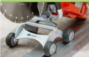
5. Place the Sawtrac carriage unit into track/guide so it is gently directed along the front edge.
